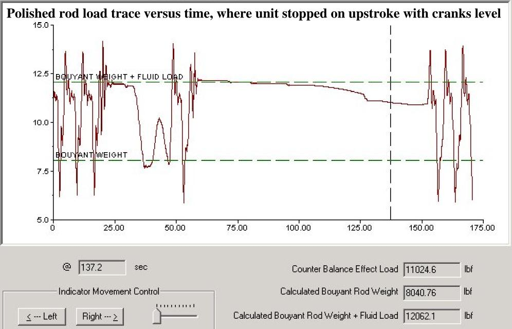
**Determine Mechanical Net Gearbox Torque Defined by API Standard 11-E**
