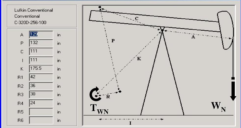
**Torque due to Polished Rod Load Net well load is:**  $W_N = net well load = (W - SU)$ **Torque due to net well load is:**  $T_{WN} = TF \times W_N$ Where: W = well load at a specific crank angle SU = structural unbalance of the pumping unit (either plus or minus value) **TF** = torque factor, inches
