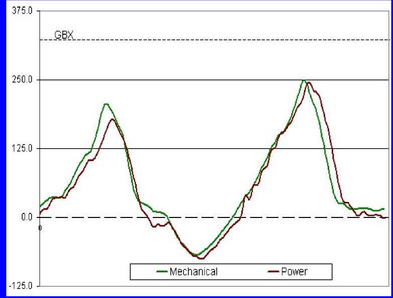
**Determine Counterbalance Moment, M, to Balance Peak Torques Between Upstroke and Downstroke**
